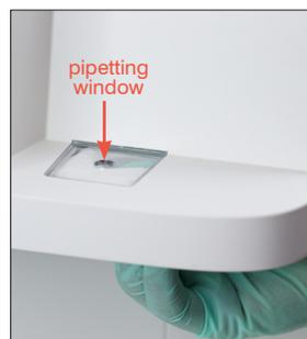
2. Open the analyser door and clean the top and bottom of the pipetting window with a damp optical tissue. Then dry with a new dry optical tissue.
