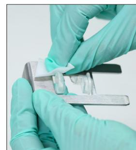
3. Remove the cartridge holder, clean it with a new alcohol prep pad, dry it with a new dry optical tissue and then set it aside.
