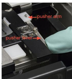
5. Press the pusher lever to the left and repeat step 4 on the right side of the pusher arm using a new rinsed alcohol prep pad.
