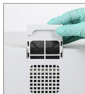
10. Remove the fan filter on the back of the analyser, rinse it thoroughly with warm water, pat it dry with a paper towel and return it to its location in the analyser.
