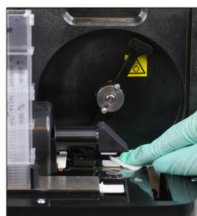
8. Using a new alcohol prep pad, clean the move arm and then dry it with a new dry optical tissue.
