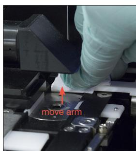
8. Using a new alcohol prep pad (not rinsed), clean the move arm and then dry it with a new dry optical tissue.
