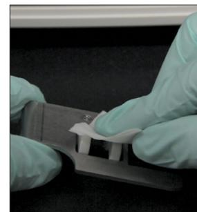
3. Remove the cartridge holder, clean it with a new alcohol prep pad, dry it with a new dry optical tissue and then set it aside.
