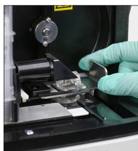
9. Return the waste bin, centrifuge shield and cartridge holder to their locations in the analyser.
