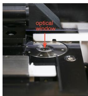
5. Using a new alcohol prep pad, clean the optical window using a circular motion (3–4 times) and then dry it in a circular motion with a new dry optical tissue.
