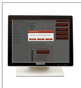
1. On the SediVue Dx Instruments screen, tap **Turn Off SediVue** and then tap **Shut Down**.
