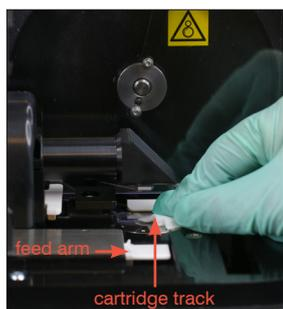
4. Using a new alcohol prep pad, clean the cartridge track and the white feed arm thoroughly. Then dry them with a new dry optical tissue.
