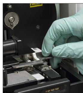
9. Return the waste bin, drip tray, centrifuge shield and cartridge holder to their locations in the analyser.
