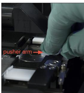
4. Using a new rinsed alcohol prep pad, clean the left side of the pusher arm five times (ensuring the right edge of the track is cleaned thoroughly) and then dry it with a new dry optical tissue.
