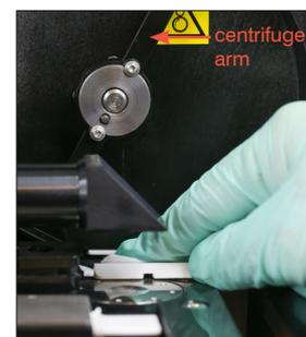
7. Gently move the centrifuge arm to the left and inspect the area below it for debris. If it's dirty, use a new alcohol prep pad to clean it and then dry it with a new optical tissue.
