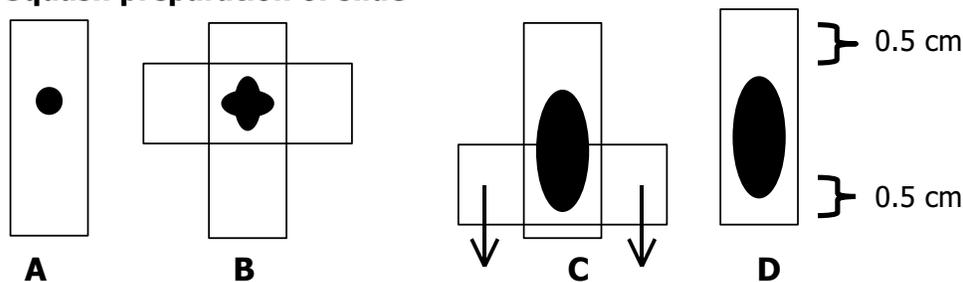
A small amount of the sample is placed on one slide and a second slide placed on top. The second slide may be perpendicular or parallel to the first. The material will spread between the two slides (**Figure 1a**). If necessary, very gentle pressure may be used to facilitate spreading (**fig. 1b**) and the top slide is gently pulled across the bottom until the two slides are separated (**fig. 1c**). The slides should slide apart, and should not be lifted away from each other (**fig. 1d**).
