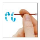
**6.** Hold the tube horizontally and roll it between your fingers for at least 30 seconds to ensure adequate staining.
