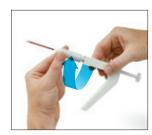
5. Hold the pipettor horizontally and unlock the barrel by twisting it clockwise. Gently remove the tube.
